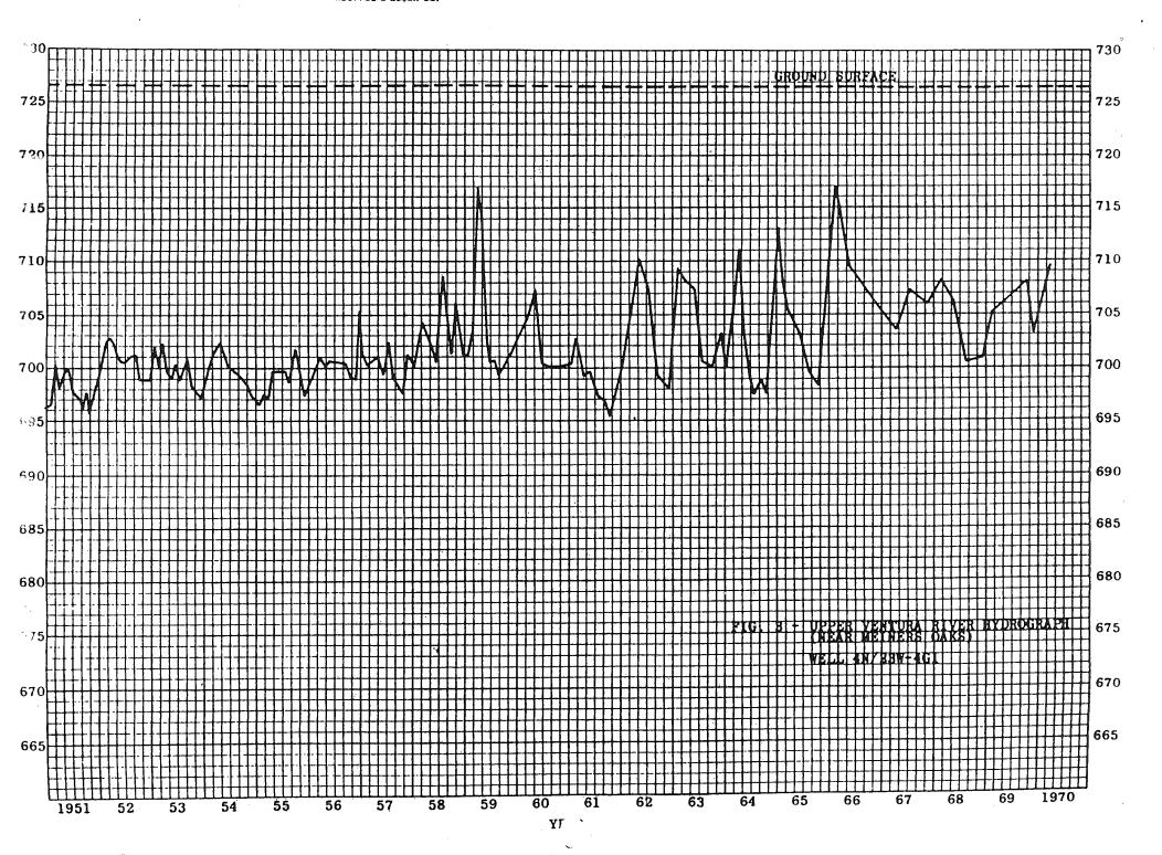
storage capacity. During periods of substantial precipitation the basin is almost immediately recharged by percolation of direct precipitation and runoff through very permeable materials. Maximum lowering of water levels occurred during a 10 month period in 1960 when a decrease of almost 125 feet was recorded. Declines of this magnitude are indicative of heavy pumpage and limited storage capacity.
